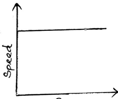
The object is moving with a uniform speed and zero acceleration.
